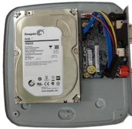
Step 3 Turn the device upside down and then secure the screws firmly.
