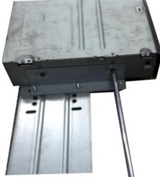
Step 7 Put the bracket back. Please adjust the CD-ROM to the proper position so that the button of the front panel is directly facing the pop-up button of the CD-ROM.
