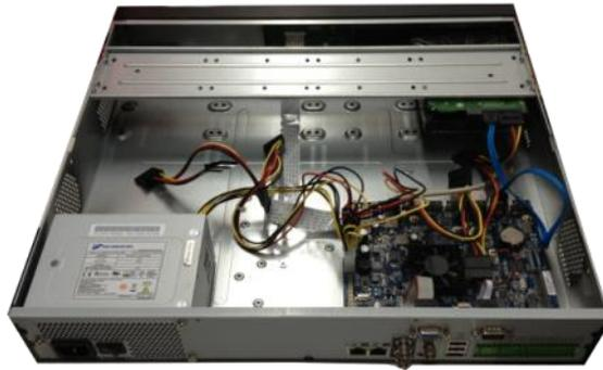
Step 4 After connect the cable, put the front cover back to the device and then fix screws of the rear panel.
