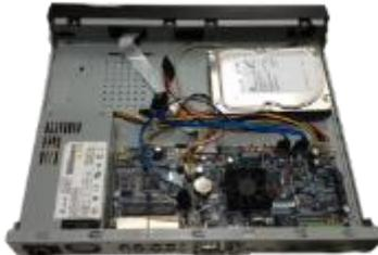
**Step 3** Turn the device upside down and then secure the screws firmly. It is to fix the HDD on the chassis.
