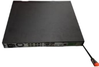
**Step 2** Place the HDD in accordance with the four holes in the bottom.
