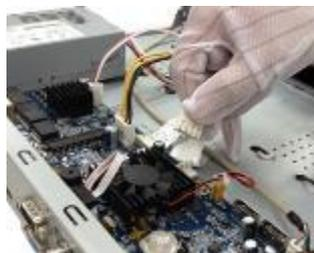
Step 3 Connect the other end of the HDD data cable and the power cable to the HDD.
