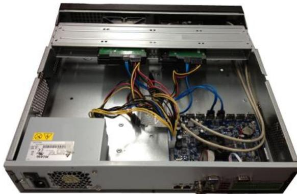
**Step 4** After connect the cable, put the front cover back to the device and then fix screws of the rear panel.
